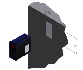
Fix the unit securely with the blocks supplied.
