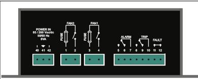
The 1048 RS485 control unit has UNIVERSAL POWER SUPPLY, it can be supplied by 85 to 260 Vca-Vcc, 50/60Hz irrespectively of polarity in Vdc (terminals 40-42). The ground must always be connected to terminal 41.
