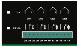
TCK SENSORS. Each temperature sensor TCK has a yellow conductor (+) and one red (-), connect the sensors following the image, example CH1 = 15 Red – 13 Yellow.
