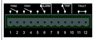
RELAYS. Output relay with 10A-250Vac-res COSΦ=1 contacts.
