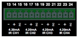
4 inputs 4.20mA for TIR409 sensors (1,5mm<sup>2</sup> section max).
