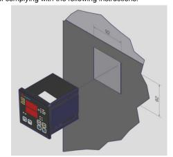
Fix the unit securely with the blocks supplied.
