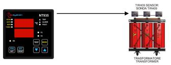
The 4.20 mA output of each TIR409 sensor must be connected to the 4.20 mA input of the relevant NT935 IR control unit input channel.
