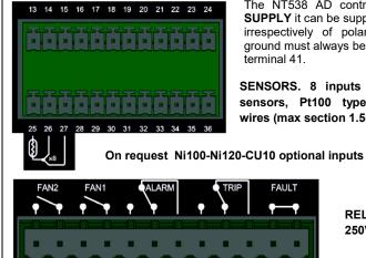
The NT538 AD control unit has UNIVERSAL POWER SUPPLY it can be supplied by 24 to 240 Vac-Vdc, 50/60Hz irrespectively of polarity in Vdc (terminals 40-42). The ground must always be connected to terminal 41.
